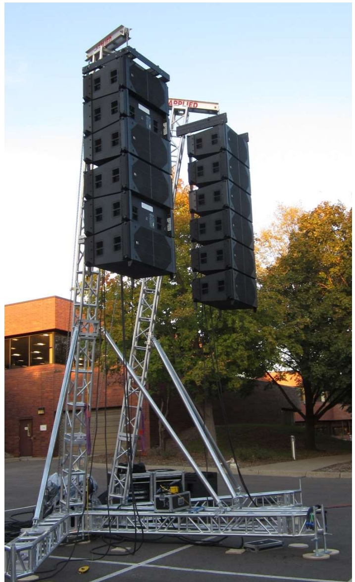
Figure 18: Testing X2 line array with the X12-125F in cardioid configuration. The cardioid presets are designed to sound the same as the standard presets on axis.
