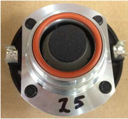
Figure 12: ND2R compression driver. The phase plug was redesigned to be an annular ring exit design.
