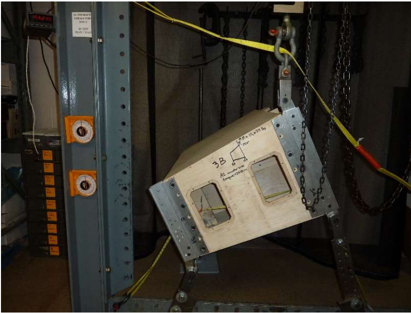
Figure 19: Structural testing of the X12-125F subwoofer system. All structural components are extensively tested on EV's pull test machine to ensure safe overhead suspension.
