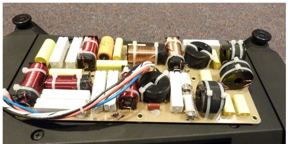
Figure 15: X1 passive crossover. Shown on top of an X1 for size reference.
