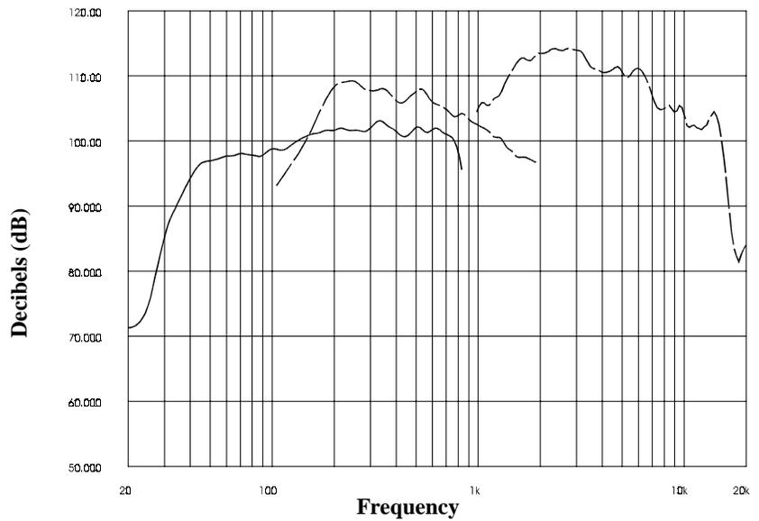
Figure 4—Variplex™ Typical Frequency Response with DX34A Digital Speaker System Processor Presets (swept sine-wave input, under anechoic environment; normalized response, from 4 volts at 500 Hz at 10 ft., with the microphone axis coincident with the aiming point, midway between mid- and high-frequency horn).
