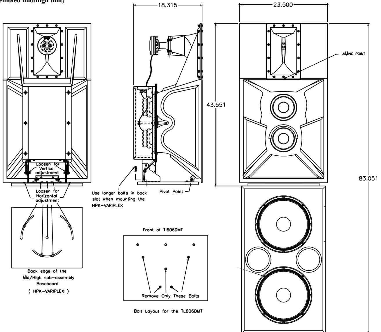
Figure 2—Aiming the Variplex™
