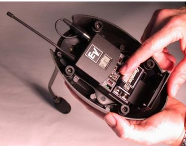
**Programmability & changing batteries are facilitated without removal of transmitter from the satellite base**
