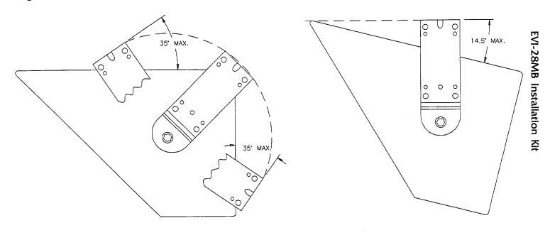
Figure 3—EVI-28MB Mounting Bracket
