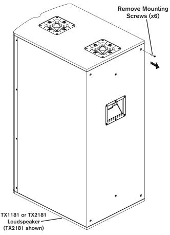
Figure 1: Remove Bolts from Rear Panel of Loudspeaker
