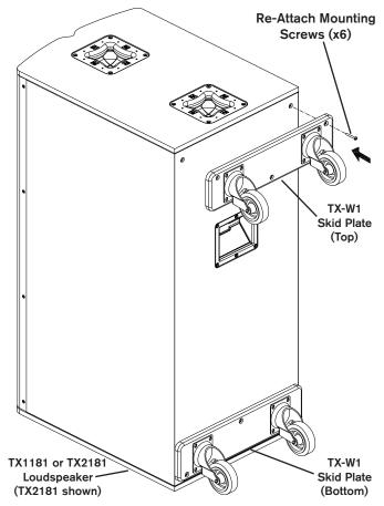
Figure 2: Align holes and Tighten Bolts
