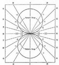
FIG. 2. — BIDIRECTIONAL POLAR PATTERN Indicates the output in decibels versus angle of pick-up.
