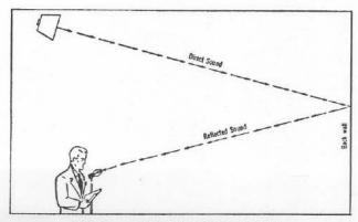
FIG. 3. — TILTING MICROPHONE REDUCES ACOUSTIC FEEDBACK
