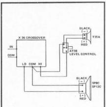
FIGURE 4 Two-Way System Wiring
