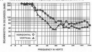
FIGURE 4 — T252 Directivity vs. Frequency, Whole Space (anechoic)
