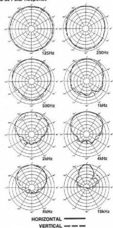
FIGURE 3 — S-80 Beamwidth vs. Frequency (whole space anechoic environment)
