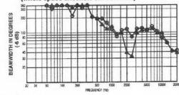
FIGURE 4 — S-80 Directivity vs. Frequency
