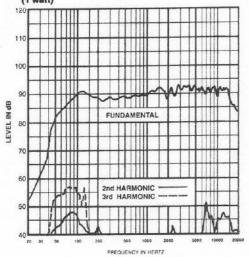
FIGURE 6 — \$-80 Harmonic Distortion 0.1 Rated Power Input (10 watts)
