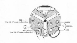
FIGURE 5 - Changing Impedance Connections
