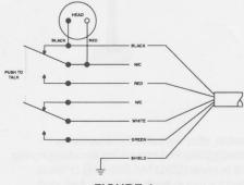
FIGURE 4 Wiring Diagram US637A/US637BA
