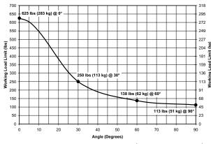
Figure 1: Suspension Point and Load Angles
