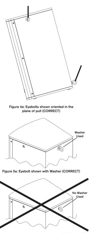
Figure 5b: Eyebolt shown without Washer (INCORRECT)
